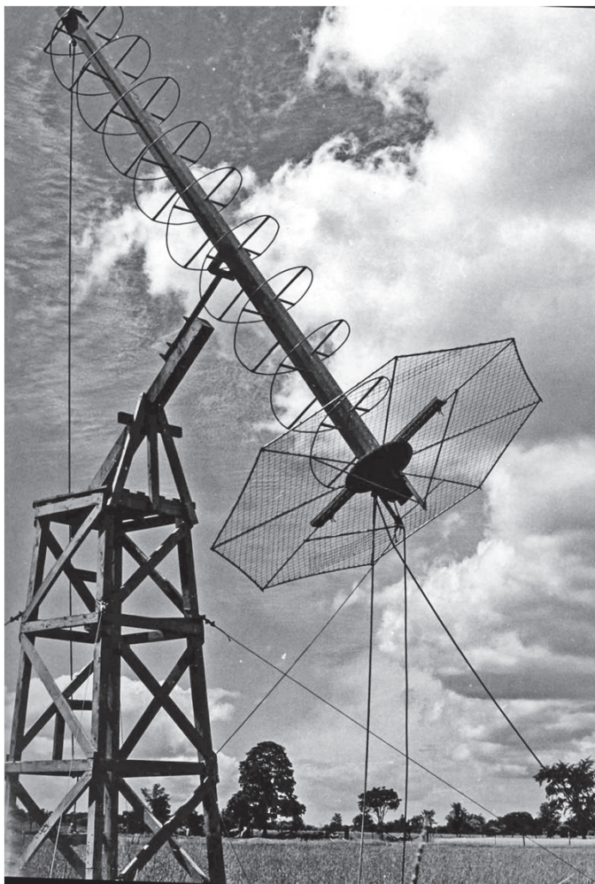
Figure 2 — David E. Hogg's MSc project—studying transient bursts of radio noise from the Sun by scanning repetitively in wavelength from 3.4m to 2.3m at 5-second intervals. The antenna is an equatorially mounted 9-turn helix of length 6m, with a reflector of diameter 3m. The receiver output is recorded directly from an oscilloscope screen by a camera.
