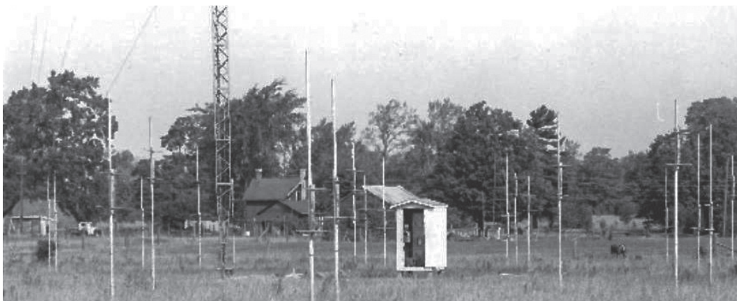
Figure 3 — The reflection-array telescope for 2-m wavelength in 1964. The two-element Yagis are reflecting elements mounted on 5-m poles for height adjustment. Through the door of the small hut can be seen the rack of receiver electronics. At 53-m height, the tower (base visible here) is an aviation hazard and has to be painted in red and white bands, besides carrying a red light at the top.
