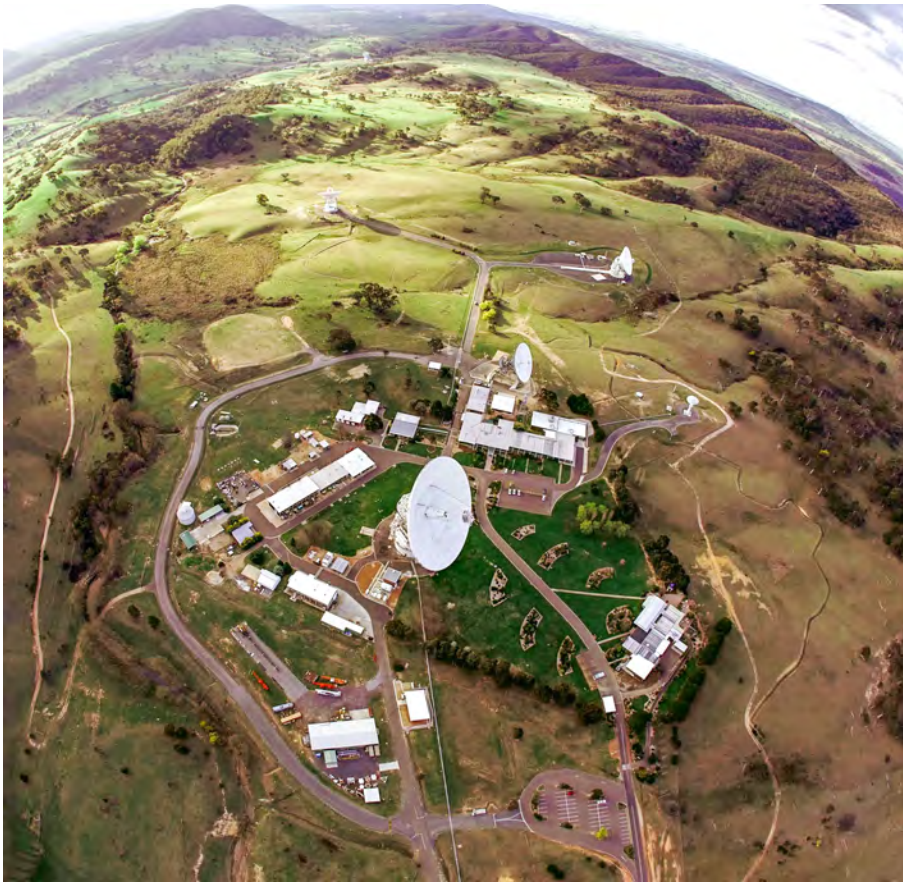
Figure 1 — Aerial view of the DSN complex near Canberra, Australia, with a 70-m antenna at the centre of frame and 34-m antennae in the background.
