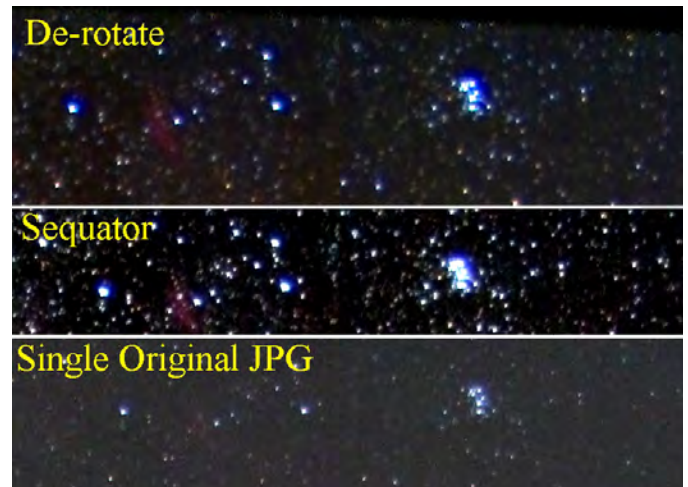
Figure 7 — A comparison of star shapes at the very top-right edge of the frame. The single image shows lens aberrations at the most open f/3.5 of this relatively inexpensive Opteka 6-mm fisheye. The de-rotated approach is nearly perfect, while Sequator’s handling is only slightly inferior (I did not spend time trying to make the backgrounds identical, since their stacking and curve processing are different). As long as the Sequator image is viewed on-screen or not overly enlarged, the result is quite pleasing. The comet at right is 46P Wirtanen.
