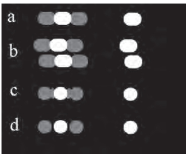
Figure 3 — Schematically trailed stars (a), copied to de-rotated positions ahead and behind, here vertically displaced to reveal the offsets (b), then compositing them with darken (c). The “true” field (d) is not completely recovered.
