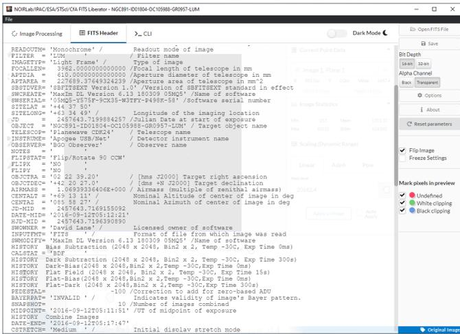
Figure 2 — Viewing the FITS header and metadata for the loaded image file.
