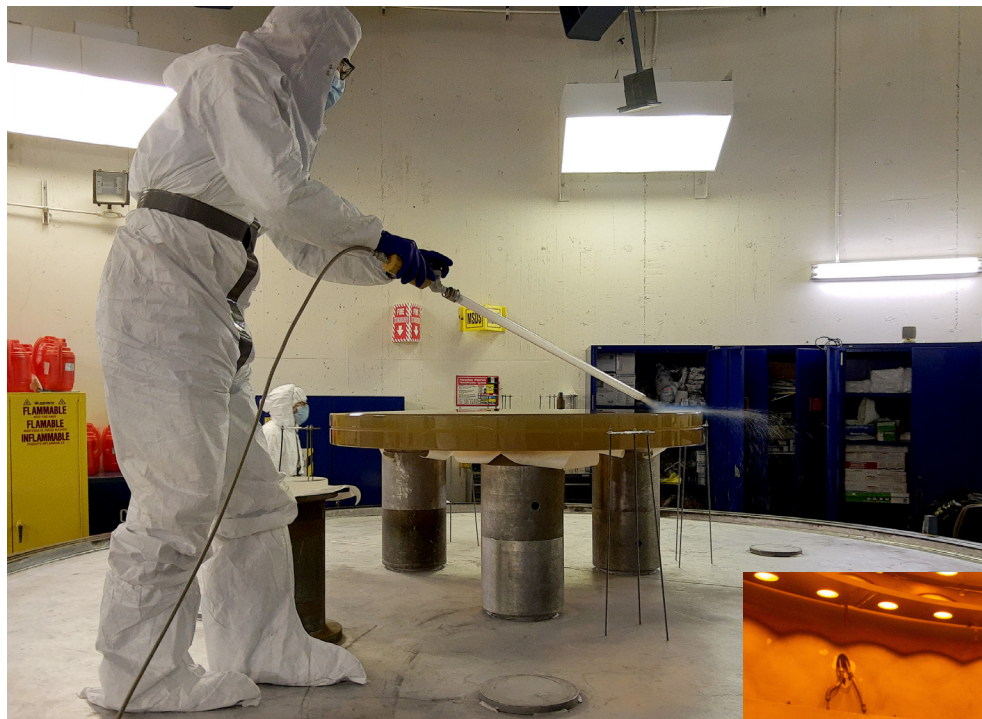
Figure 1 — CFHT staff use carbon dioxide snow to clean off the surface of the secondary mirror.
