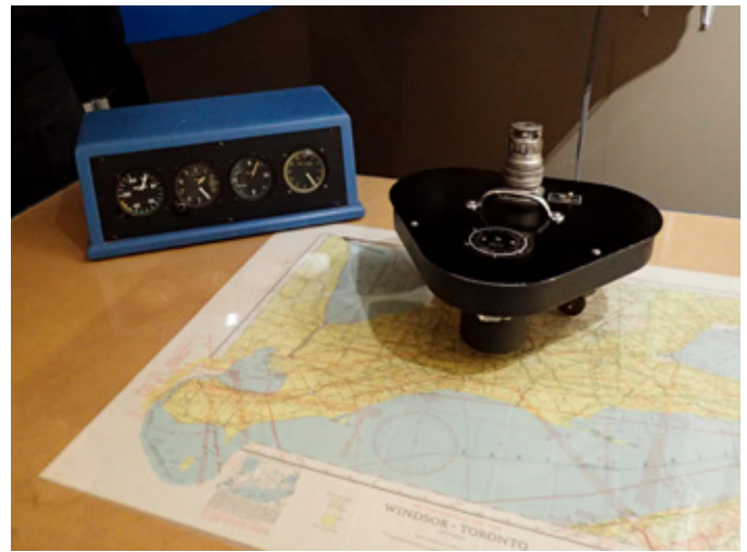
Figure 2 – The crab of the Link trainer at the Canadian Warplane Heritage Museum. It would have been connected to the aircraft portion by a cable. Photo by the author.
