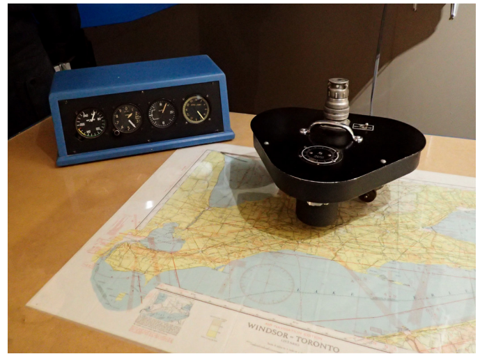
Figure 2 – The crab of the Link trainer at the Canadian Warplane Heritage Museum. It would have been connected to the aircraft portion by a cable. Photo by the author.
