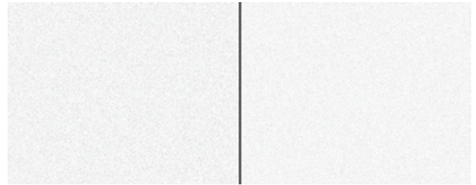
Figure 2 – Image on the left has an SNR of 27 dB while the image on the right has an SNR of 30 dB.
