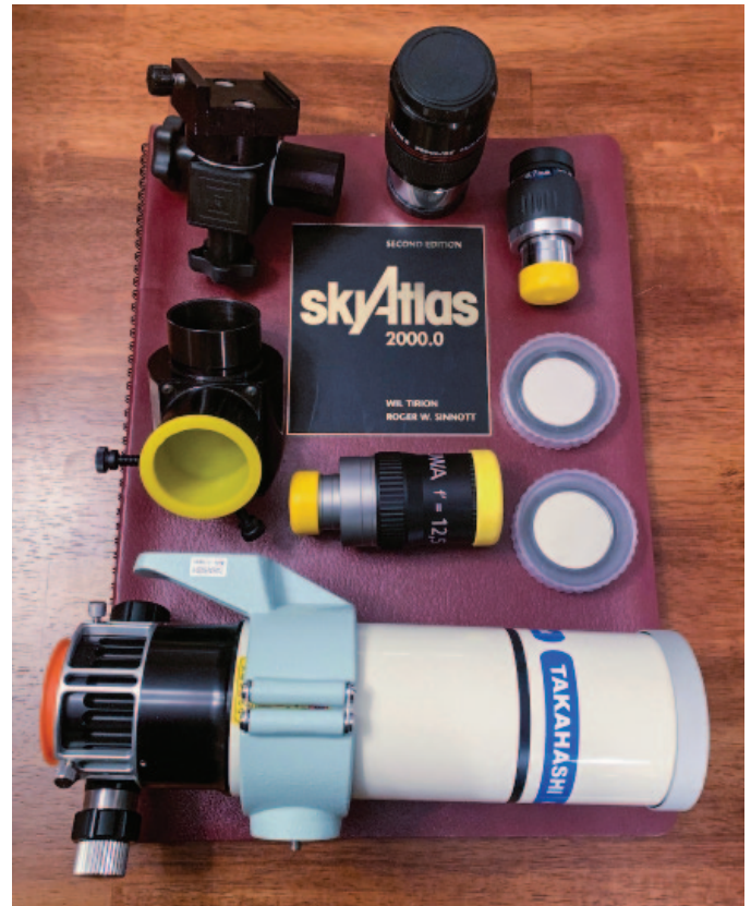
Figure 1 — The tiny Takahashi FS60 and an assortment of wide-field eyepieces and all the accessories needed for a night under the stars. Image by the author.
