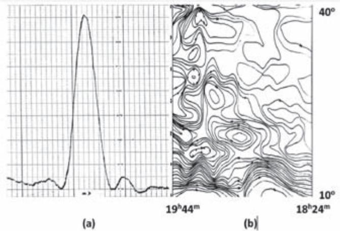
Figure 7 — (a) Chart recording at 2 metres by Hesse, as *Cas A* transits through the NS fan beam power pattern of the long arm of the moving-tee telescope. Chart speed is one large division per 15 minutes; hence the fan beam is  $1^\circ$  EW at half maximum. Sidelobes are visible on each side, of about 5%.
