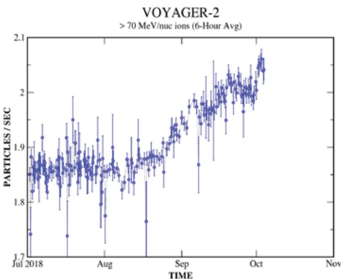
Figure 1 — A graph of high-energy particle detection rates acquired aboard the *Voyager 2* spacecraft up to early October. The PGH rate consists of >70 MeV/nuclei ions, primarily protons, and is a good indicator of the level of modulation of galactic cosmic rays. It can also respond to large solar flares.
