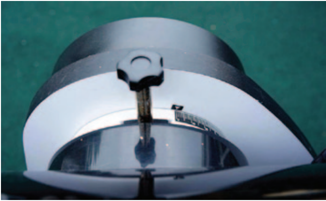
Figure 3 — The altitude axis has a scale for leveling the tube before initialization.
