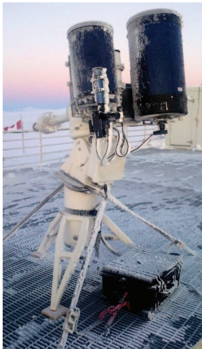
The Ukaliq autonomous site-testing telescope setup on the PEARL rooftop seen dusted with frost, just at sunrise after one long “night” of observing Polaris.
