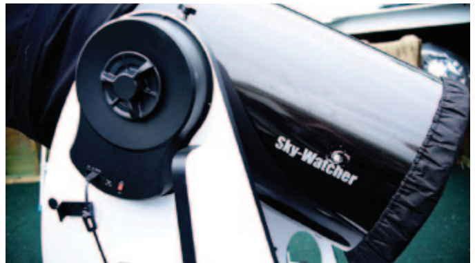
Figure 2 — The larger Sky-Watcher dobs have adjustable bearings on both axes.
