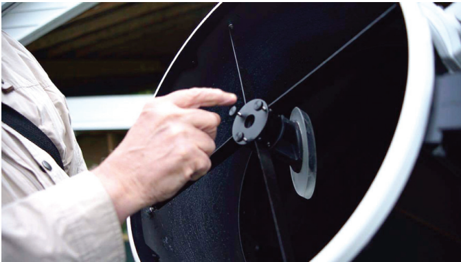
Figure 4 — Consider replacing the secondary mirror adjustment hex-screws with knobs to eliminate the need for a tool.
