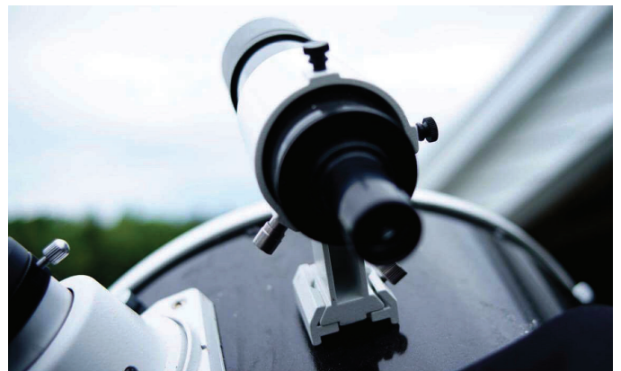
Figure 5 — Take the time to align the finder with the telescope before initializing the electronics.
