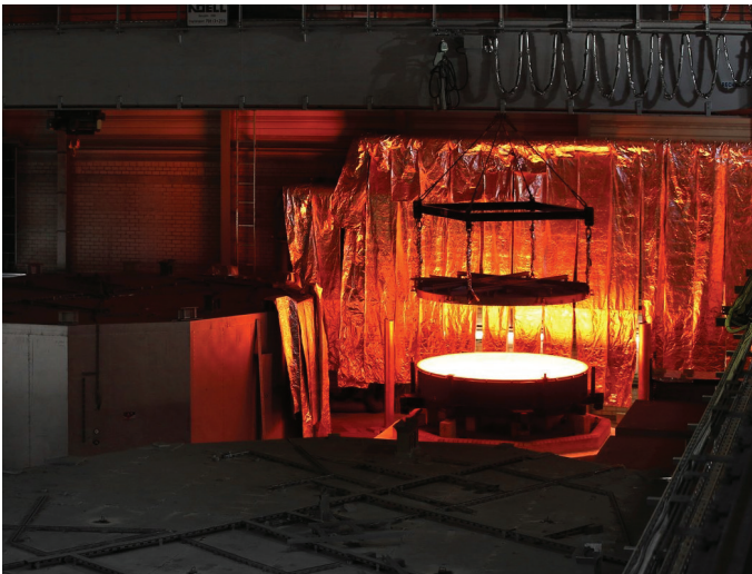
Figure 2 — Opening of the ELT secondary mirror blank mould, containing the still very hot ZERODUR® glass at first annealing. The blank was transferred from the SCHOTT melting facility to the SCHOTT 4-metre blank annealing facility in Mainz, Germany, in May. The casting of this mirror is a major step toward building the world's biggest eye on the sky, one of ESO's greatest feats. Image: SCHOTT/ESO
