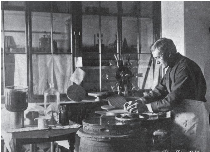
Figure 2 — The large mirror during fabrication is shown on a barrel with a worker. Note the notches chiselled on the side of the glass. The mirror cell can be seen in the background leaning against a window. Photo: Scientific American , 1903 January 24.
