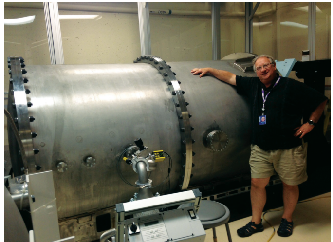
Figure 2 — SPIRou cryostat at NRC, with DAO director Dennis Crabtree to show the scale.
