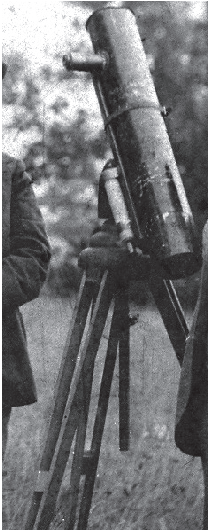
Figure 3 — Detail from a photograph of a Society “star party” ca. 1900, showing an amateur reflector contemporary with Sir Adam’s now lost instrument (the instrument shown here probably had a 10.8-127 cm primary mirror, whereas Sir Adam’s was equipped with a 15.2 cm mirror). Reproduced courtesy of the RASC Archives.
