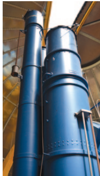
Figure 2 — The Bruce double astrograph in its original dome at the Landessternwarte Königstuhl. The guide telescope is to the left, with one astrograph clearly visible on the right, and the second slightly visible in the gap (photo by author).
