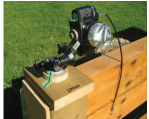
Figure 2 — The camera mounted on a tripod head affixed to a custom wooden mount that could be accurately placed on the park bench.
