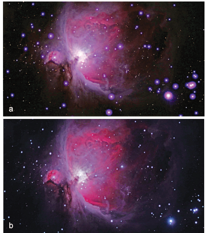
Figure 3 — (a) Image of M42 taken with the CT-152 without filter, showing bloated, red-haloed stars. (b) M42 as above, after insertion of an IDAS LPS filter, showing tighter, colour-free stars and enhanced contrast.
