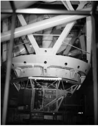
Figure 8 – Close-up view of the instrument cage under the mirror of the 200-inch telescope from the visitor window. A portion of the massive horseshoe mount is visible at the top left.
