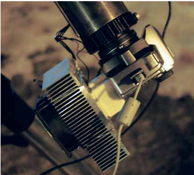
Figure 7 – The thermoelectric cooler attached to the camera.
