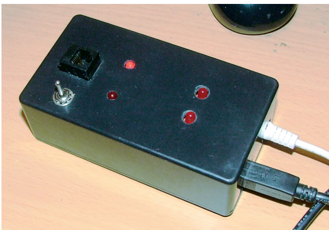
Figure 4 – The finished focuser.
