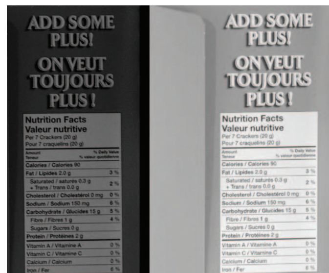
Figure 7 — Nikon D40 with 135-mm lens, f/4 , ISO 800, 1/80 -th-second shutter speed. Left: normal Bayer layer converted to grayscale. Right: camera with Bayer layer and microlens removed.
