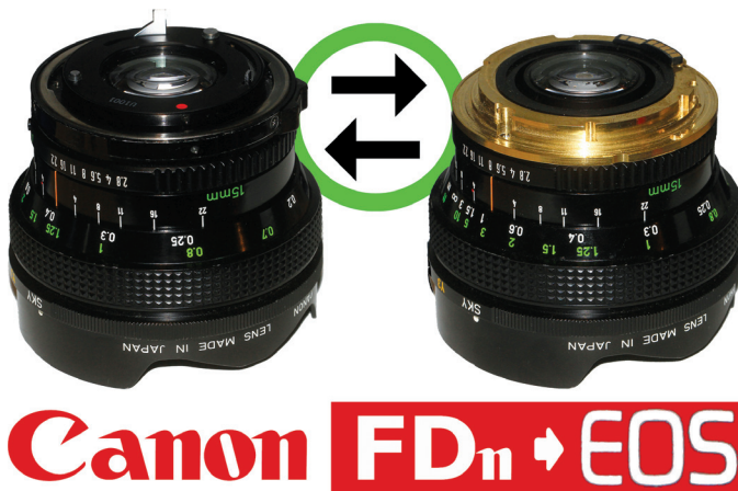
Figure 1 — A before-and-after comparison of the back mount of a Canon 15-mm f/2.8 FD lens showing the Ed Mika-modified adapter.
