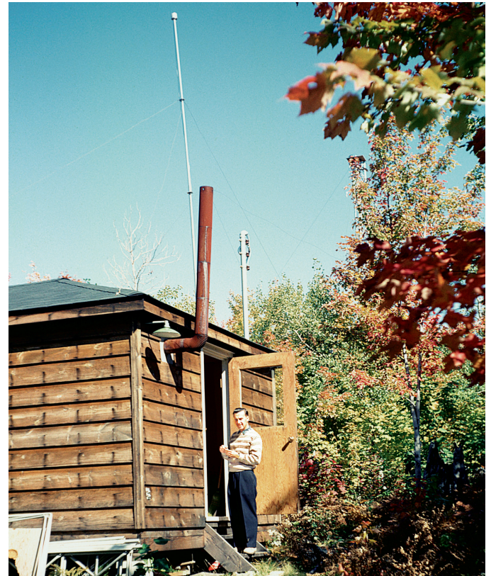
Figure 2 — Technical Assistant Anatol Kryworuchko enters the Dominion Observatory's cabin on the Eardley Escarpment, early autumn 1963. The long tubular shaft behind the chimney supports a weatherproof cylindrical housing for a large-diameter photovoltaic cell. A matched unit was installed on the roof of the Geophysical Laboratory on the CEF. The outputs of both cells were fed into strip-chart recorders.
