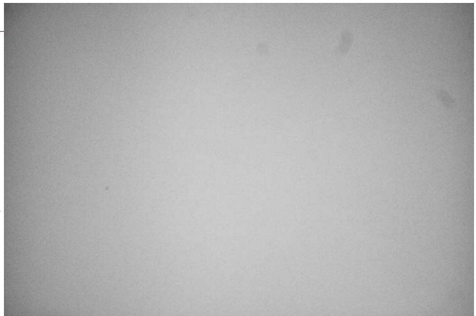
Figure 1 — A sample flat frame, showing vignetting in the corners of the optical system and the shadows of dust spots in the camera.
