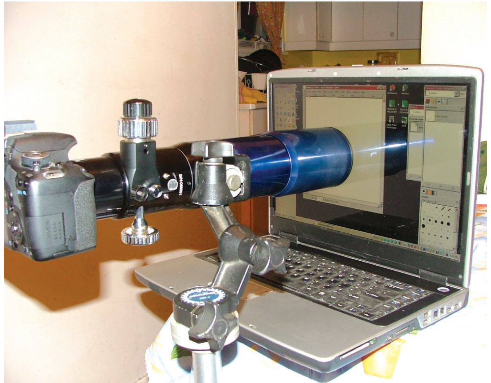
Figure 4 — Shooting flat frames using a computer screen.
