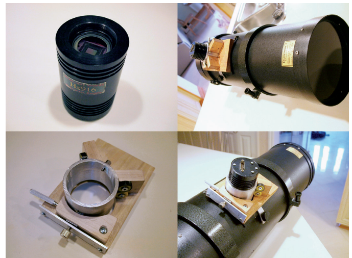
Figure 4 — Stages in the construction of the Schmidt camera's new focuser and camera mount.
