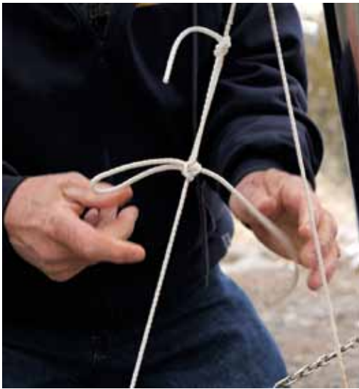
Figure 4 – Tie off the two ends with a half hitch.
