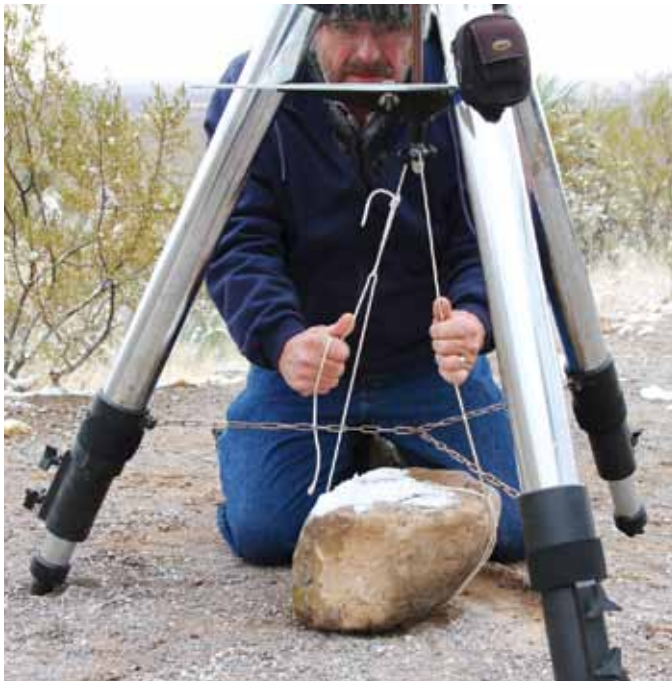
Figure 1 — Tie a loop into one end of the cord, wrap once around the rock (or pass it through the eye on the stake) and up over whatever works on the tripod. Bring the other end of the cord through the loop and pull down on it while pulling up on the other side. You now have a two-to-one advantage, as if you were using a pulley. I tightened up on it until the rock was just coming off the ground.
