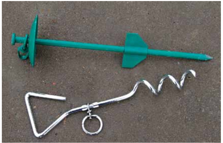
Figure 5 – Above is the pet stake, beneath it is the spiral tent stake. Either would work well in firm soil or clay, but if you use the pet stake you'd better have something to pry it out with when you're done!
