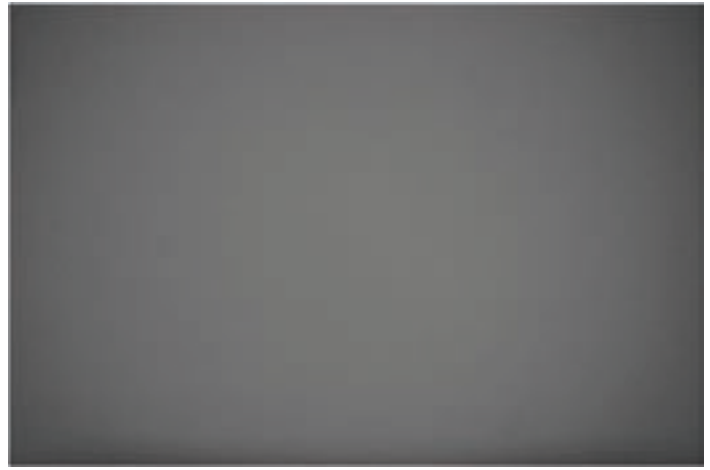
Figure 5 — Flat-field image. Note the effects of vignetting.
