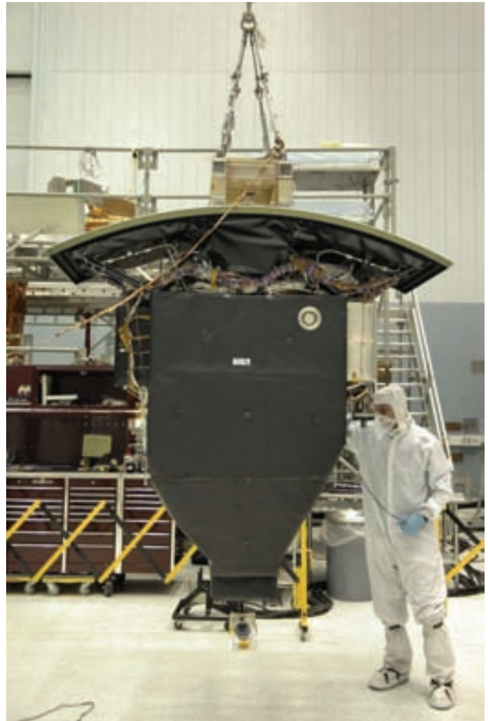
Figure 1 – The latest in space cameras: Hubble's Wide Field Camera 3 in the clean room prior to launch and installation. Image: NASA
