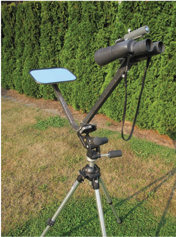
Figure 1 – The Binocular Mirror Mount (Mark 2). Set the eyepieces to a convenient height and aim by tilting the mirror. The frame is one leg of an old barbeque. A barbeque has four legs so you have four tries at getting it right.
