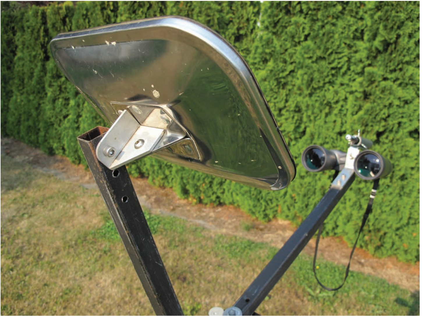
Figure 3 – Both the mirror and the frame show evidence of a former life. They are bolted together with a short piece of angle, cut and filed to suit.
