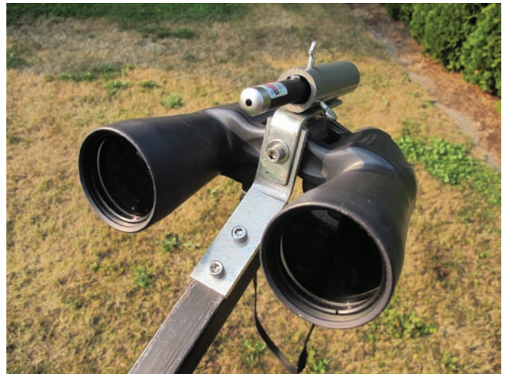
Figure 2 – The green-laser bracket is a nice little project in its own right and has many uses for aiming binoculars or telescopes or even cameras. It is mounted on a standard hardware-store repair angle. The binoculars and laser together bolt to the frame with a purpose-made bracket.
