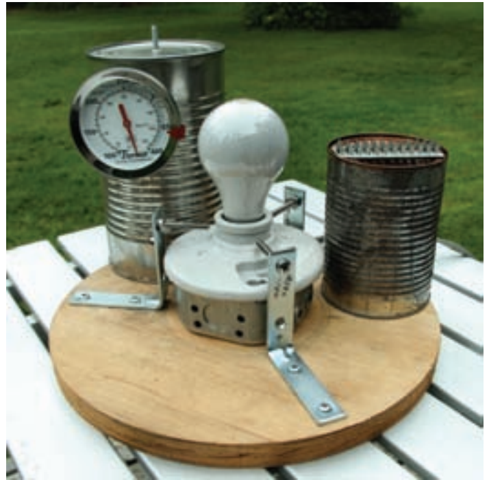
Figure 1 — The three main components of the desiccant oven. That metal thing under the lamp base is an octagon box. It's not really optional because it provides a fireproof enclosure for your electrical connections.
