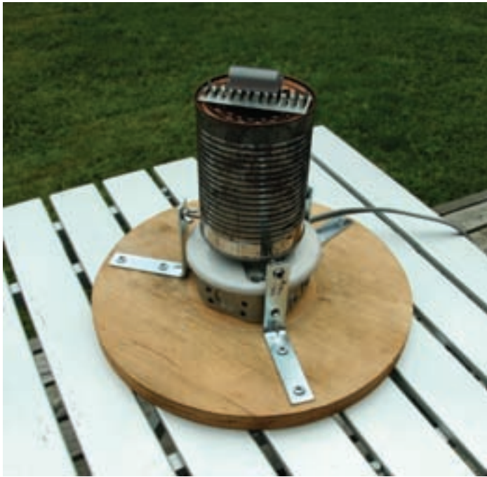
Figure 2 — The inner can in place. Note the double row of holes around the perimeter of the top. The holder for the desiccant plug could be cut and bent out of a tin can. It doesn't need to be fancy, just needs to allow airflow around the plug.
