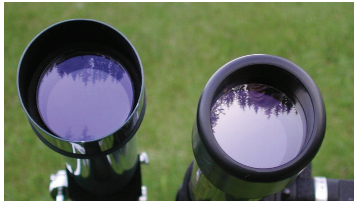
Figure 3 — Superior coating on the older glass (left) results in a dimmer reflection and better light transmission.
