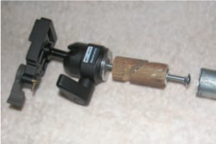
Figure 3 — The wedge assembly. The most difficult part of this is drilling the hole exactly down the centre of the dowel. It wants to go off to one side or the other. Use a centre punch (or a nail) to make a dimple and drill half in from each end. Keep trying till you get it right. Our broom handle is a lot shorter now.
