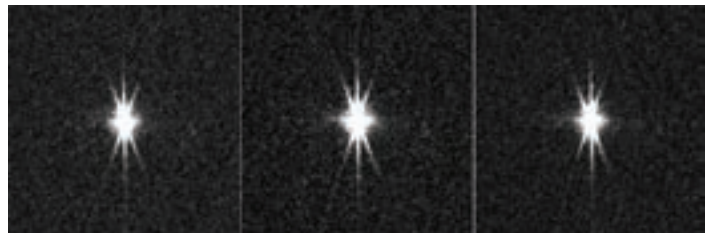
Figure 2 — Left: inside focus .015"; middle: at focus; right: outside focus .015"
