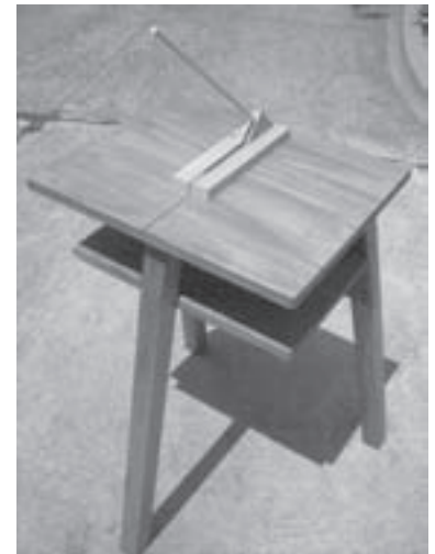
Figure 3 — A gnomon for polar alignment.
