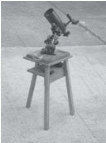
Figure 1 — The tabletop mount with a 100-mm Maksutov-Cassegrain on the three-leg table.
