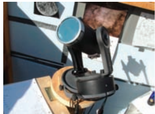
Figure 9 — White-light telescope used for solar observations
