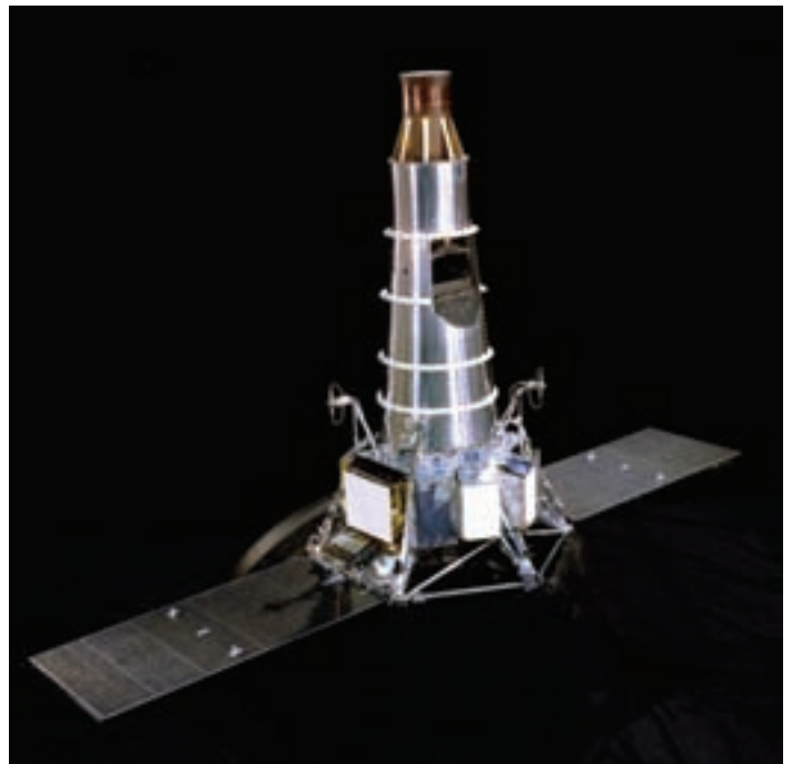
Figure 5 — Ranger 7 spacecraft, launched on 1964 July 28 and arriving at the Moon three days later. The spacecraft carried six television cameras, sending back high-resolution photographs of the lunar surface until its impact in an area between Mare Nubium and Mare Cognitum. NASA image.
