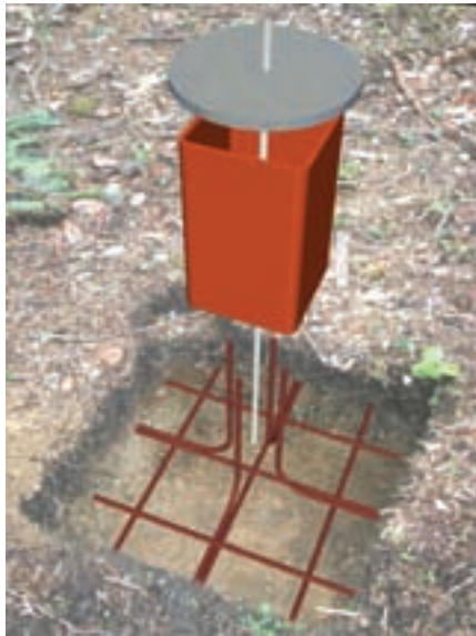
Figure 1 — This image shows the arrangement of the rebar. The tube has been raised and made shorter for clarity.
