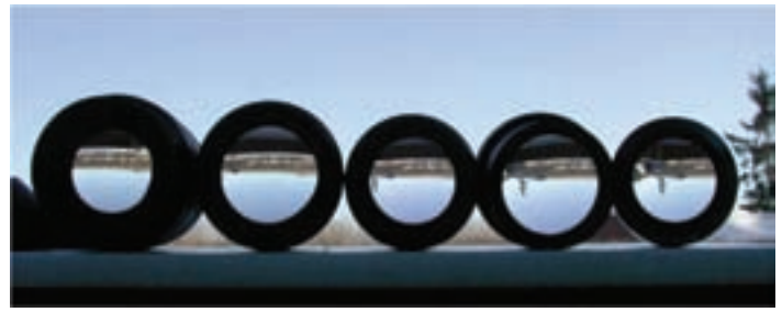
Figure 2 — No squinting here: All of these 2-inch format eyepieces have large eye lenses and multi-coated optics.
