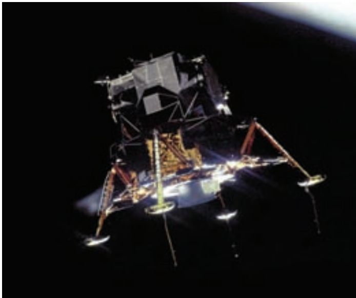
Figure 1 — The Apollo 11 Lunar Module “Eagle,” in a landing configuration as photographed in lunar orbit from the Command and Service Modules “Columbia.” Image: NASA
