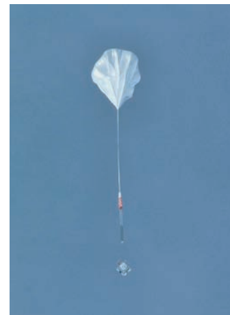
The ATIC cosmic-ray detector ascends to the stratosphere tethered to a high-altitude research balloon. Image: NASA.
