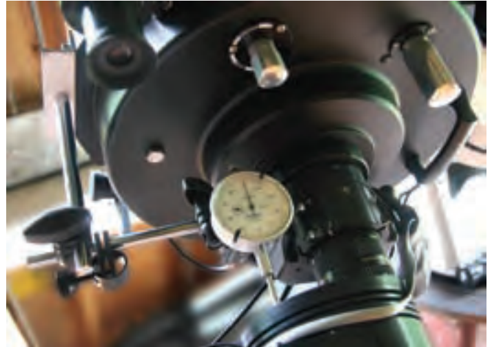
Figure 1 — The dial gauge fitted to a Schmidt-Cassegrain telescope.
