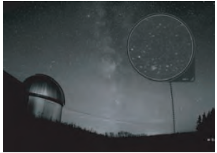
Figure 3 — Thirty-second exposure taken with a Canon 20Da and a 15-mm fisheye lens at ISO 1600 that shows undersampled star images. The highlighted circular region shows a portion of the image zoomed to show actual pixels. This image shows the Milky Way and the University of Manitoba’s Glenlea Astronomical Observatory.
