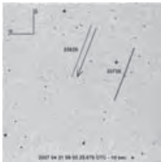
Figure 2 — A CASTOR image of two Russian " Glonass " GPS (MEO) satellites (CASTOR #s 0558 and 0559; NORAD #s 23735 and 23620 respectively) obtained with the NexStar 8i telescope and SBIG ST-9XE CCD. The compass directions indicate increasing Right Ascension and increasing Declination. The arrow indicates the direction of travel of both satellites.
