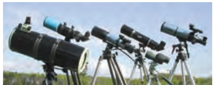
Figure 1 — left to right: Generic 8-inch f/4, above it, Stellarvue 80-mm f/6, Sky-Watcher 70-mm f/7, Sky-Watcher Equinox 80-mm f/6.25, Accuter Kolibri 750 monocular, and Sky-Watcher 80-mm f/5
