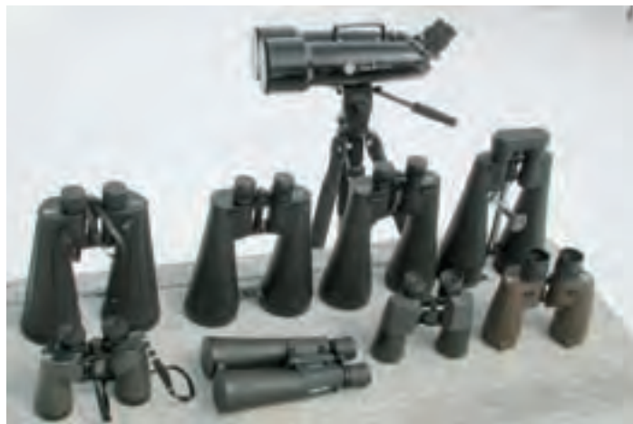
Figure 1 — Some of the binoculars examined. Front row left to right: Bushnell Explorer 7 \times 50, Meade 9 \times 63 roof prisms, no-name 10 \times 50, William Optics 7 \times 35 ED. Back row: Meade 11 \times 80, Antares 11 \times 80, Omcon 15 \times 80, Nova 20 \times 90 triplet objectives. Olivon 20/40 \times 100 on optional tripod.
