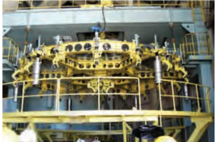
Figure 3 — The mirror support mechanism at Subaru, designed to support the 8-m glass during its travels from the telescope to the washing and realuminizing tank.
