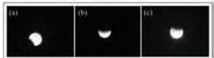
Figure 4 — The three "raw" partial-eclipse images analyzed in order to estimate the radius of the Earth's shadow at the Moon's orbit. Each image was greatly enlarged in turn and analyzed according to the construction described in Figure 3. All images were taken from Regina, Saskatchewan, at the times indicated in column 1 of Table 1, with a Sony 8 Handycam operating in single-frame-capture mode.
