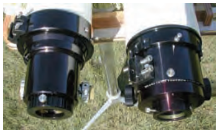
Figure 2 — AP (left) has a 2.7" rack-and-pinion two-speed (10-to-1) focuser, while the TMB (right) has a 3.5" rack-and-pinion two-speed (10-to-1) rotatable focuser.
