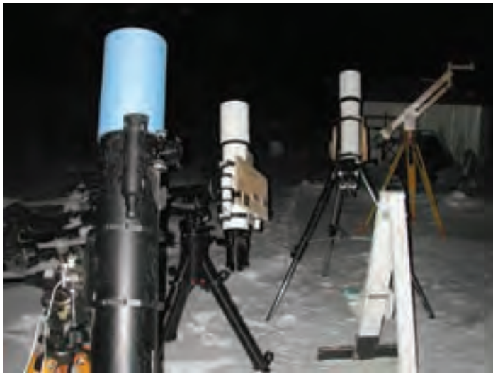
Figure 3 — Three frosty tubes lined up in the snow at -28 °C. The 150-mm Maksutov Newtonian (left) is my main planetary telescope, and was used as the control to evaluate seeing conditions and Martian detail. The TMB on a Losmandy G-11 mount (centre) is a nice sturdy combination, while the AP (on the right) on a relatively sturdy alt/az mount proved to be a bit frustrating for high-powered planetary observing. Mars is high overhead.
