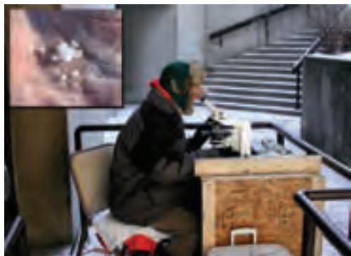
Figure 4 — Ron Peterson studies the natural occurrence of the newly discovered magnesium sulphate mineral, meridianiite (inset), in an outdoor setting at Queen's, keeping it stable below 2 °C.
