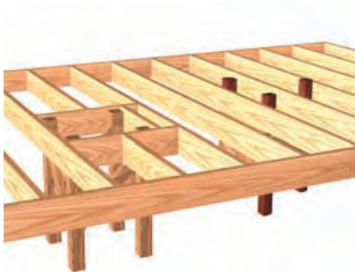
Figure 2 — Joists and framing. Use joist hangers and galvanized nails to frame the opening for the Dob base.
