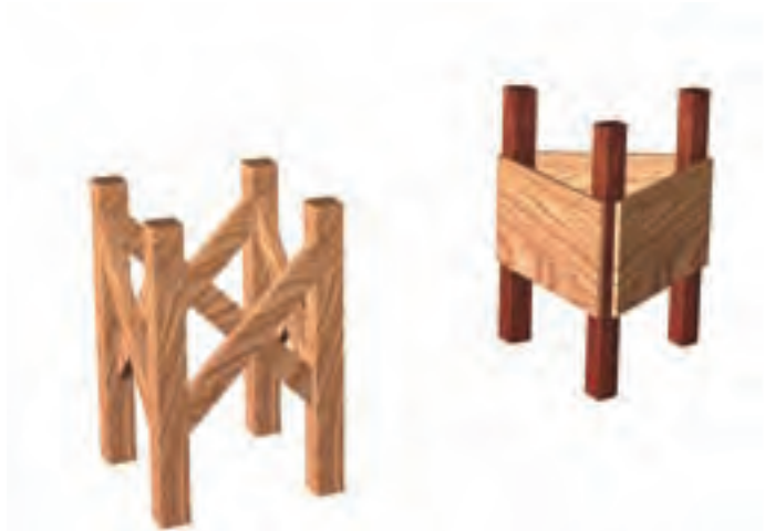
Figure 1 — Dob and tripod bases. Both the Dob base and the tripod base can be preassembled. Use braces to stiffen the assembly or, much easier, a plywood skirt.
