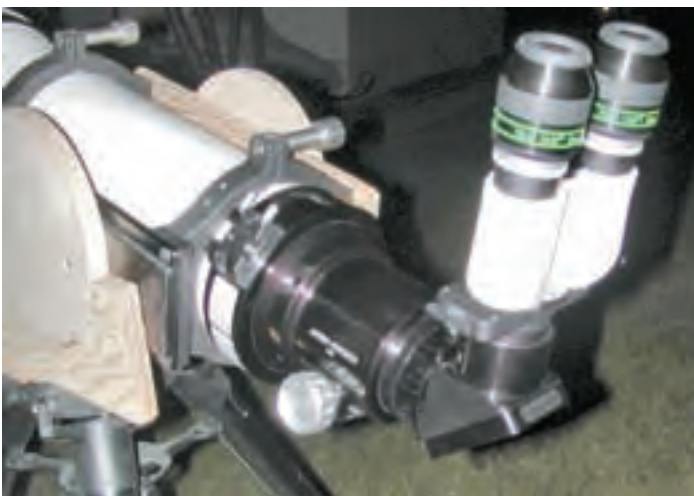
Figure 1 — A modern no-compromise binoviewing set-up of Astro-Physics 130 refractor, TeleVue diagonal, and 24-mm Panoptic eyepieces set in a Denkmeyer II binoviewer with power switch.
