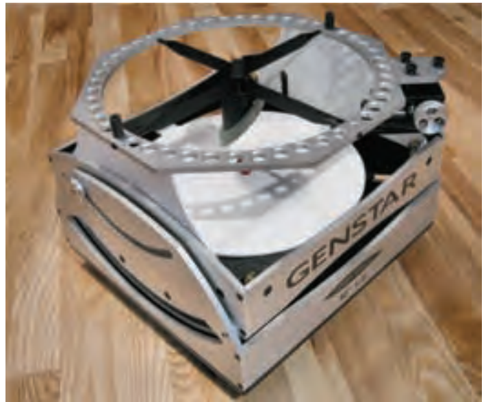
Figure 3 — The Genstar rocker box with primary and secondary mirrors secured for storage or car travel.
