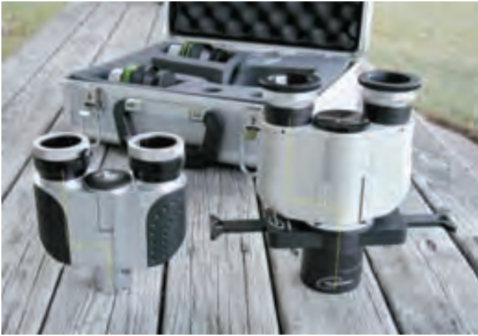
Figure 4 — Using binoviewers means adding as much as five inches to the light path (yellow line shows the altered and extended path) causing focusing and magnification problems.
