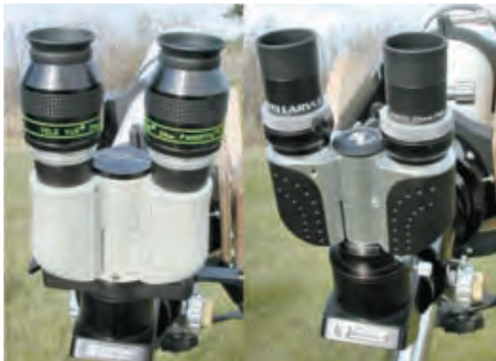
Figure 2 — The two units used in this investigation represent two trends current in binoviewing. The Denkmeier no-compromise units (left) have large prisms yielding a ~25-mm clear aperture, they are set up for use in 2-inch format at the field lens end while maintaining 1.25 eyepieces, and can use the optical correction system (OCS) — a telenegative lens (a.k.a. Barlow) that allows the unit to reach focus on telescopes with limited focal travel. The Denkmeier binoviewers are best considered as part of a surprisingly versatile and encompassing system of lenses and adaptors to optimize the binoviewing experience; these are used with TeleVue 24-mm Panoptic eyepieces to maximize their strengths. On the right is the Stellarview system.
