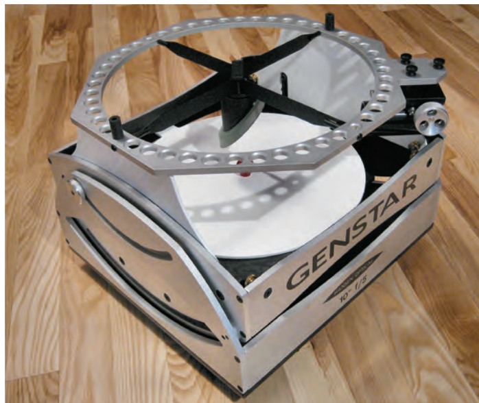
Figure 3 — The Genstar rocker box with primary and secondary mirrors secured for storage or car travel.
