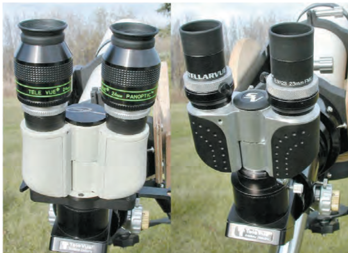
Figure 2 — The two units used in this investigation represent two trends current in binoviewing. The Denkmeier no-compromise units (left) have large prisms yielding a ~25-mm clear aperture, they are set up for use in 2-inch format at the field lens end while maintaining 1.25 eyepieces, and can use the optical correction system (OCS) — a teleneegative lens (a.k.a. Barlow) that allows the unit to reach focus on telescopes with limited focal travel. The Denkmeier binoviewers are best considered as part of a surprisingly versatile and encompassing system of lenses and adaptors to optimize the binoviewing experience; these are used with TeleVue 24-mm Panoptic eyepieces to maximize their strengths. On the right is the Stellarvue system.
