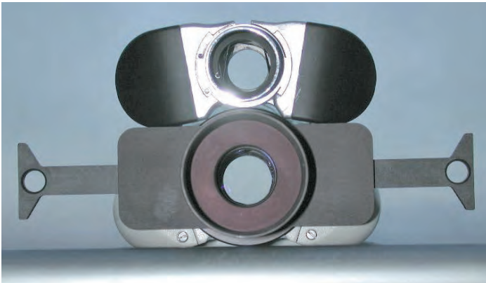
Figure 3 — This comparison shows the clear aperture, relative sizes, and the dimensions of the two prism housings. The bars on either side of the Denkmeiers are the levers that push correcting lenses into the optical path to change magnification. Note that the SVs are 1.25-inch format, while the Denkmeiers are 2-inch.
