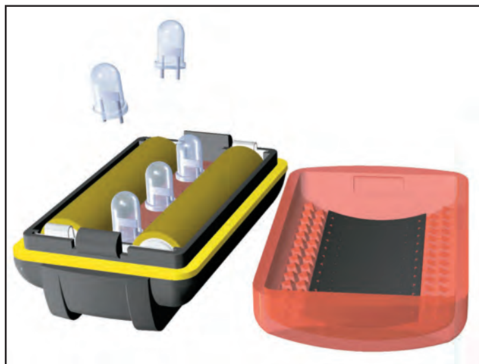
Figure 2 — Remove two of the LEDs gently with brute force. Put electrical tape up the inside of the lens and you're done.
