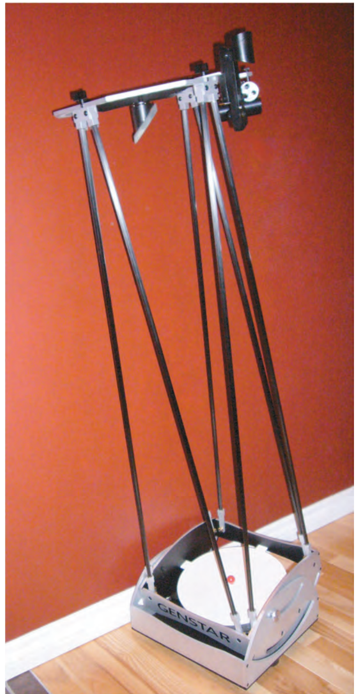
Figure 2 — The Genstar with its shroud removed in order to show the carbon-fibre truss tubes and secondary holder.
