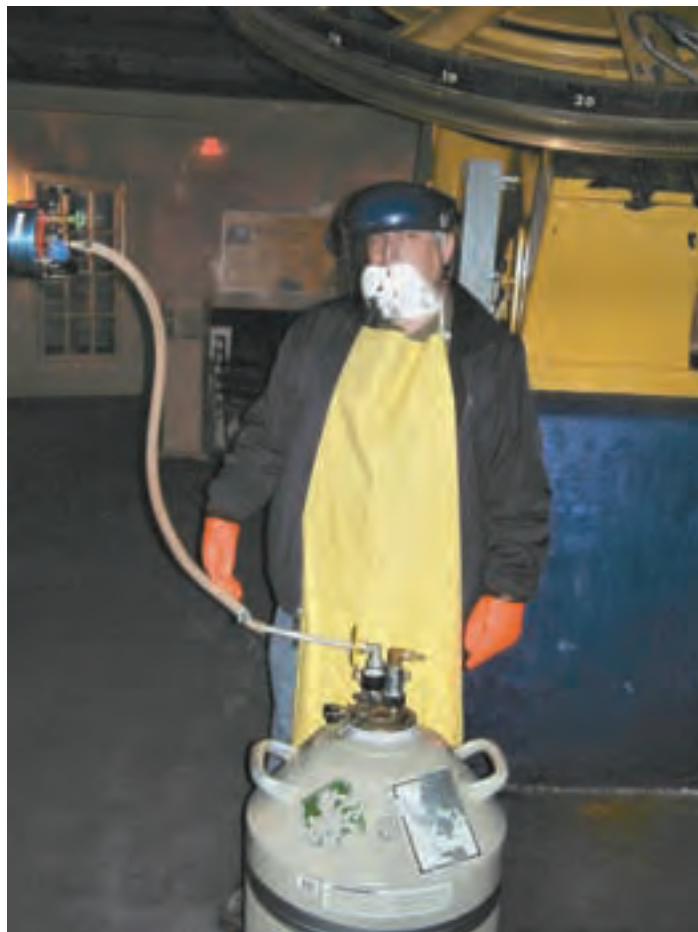
Figure 2 — Safety first! Liquid nitrogen at -110\text{ }^{\circ}\text{C} needs to be poured into the Dewar every four hours to keep the CCD camera at operating temperature. We may have been the last observers to do this since they were busy installing a continuous \text{LN}_2 circulating system.
