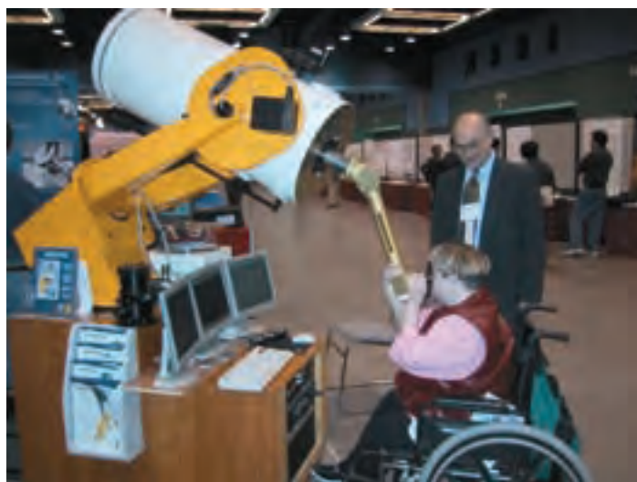
Figure 1 — An articulated eyepiece will allow wheelchair-height viewing of the Cosmos. The eyepiece attaches to the telescope and extends down to the seated stargazer.
