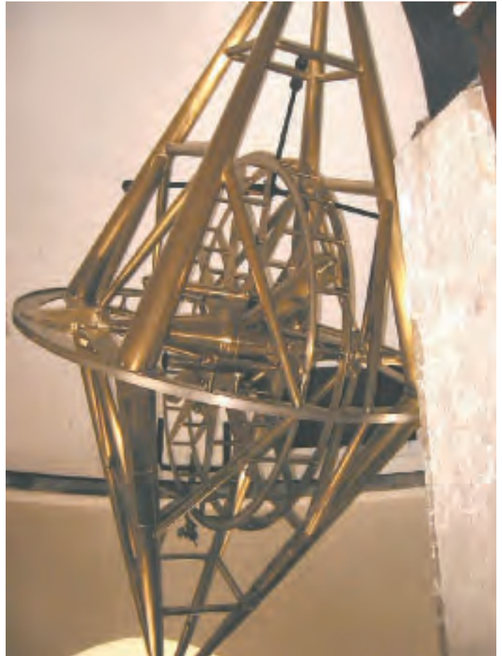
Figure 2 – Troughton 2-inch brass equatorial telescope.
