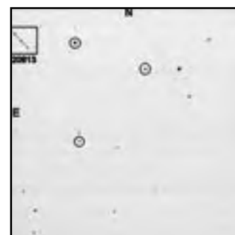
Figure 7 – Artificial satellite Molniya 3-39 (#20813) as seen by the SMARTScope facility at 05:10:35.5 UTC on December 8, 2003. The field of view is 10.0 by 10.0 arcminutes. The streak looks slightly longer in this image compared to CASTOR II's image, despite the identical exposure times, because of the smaller field of view of the SMARTScope detector.
