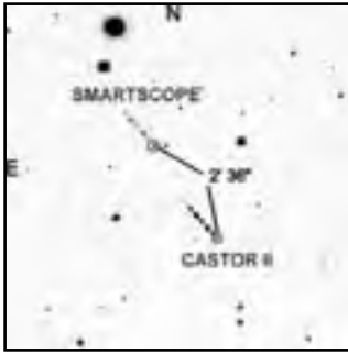
Figure 8 – The apparent positions of the Molniya 3-39 satellite as seen by both the CASTOR II and SMARTScope facilities. The SMARTScope image of the satellite was grafted onto the cropped CASTOR II image and adjusted to the CASTOR II image scale. The measured parallax angle of the satellite is indicated.
