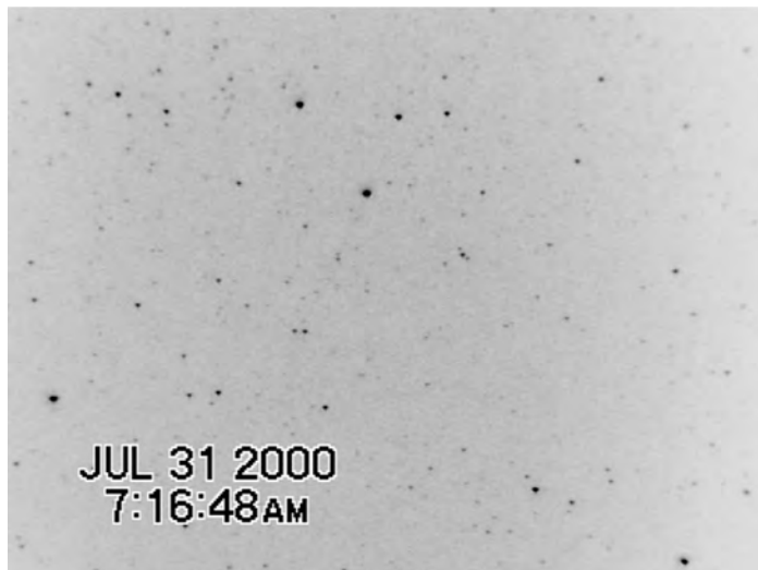
FIGURE 1 — A typical 0.033 s stellar field from one of the image-intensified CCD detection systems. On the original image, stars to about +8.6 magnitude are visible, with about 500 stars identifiable. The field of view is 14.0 degrees by 10.5 degrees. The brightest star in the upper central part of the image is the +3.6 magnitude star 41 Ari (SAO 75596).
