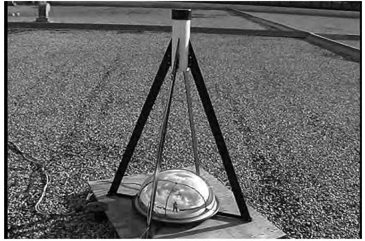
FIGURE 1. – Sandia meteor camera on the roof of Athabasca University. A video camera is housed in the vertical white tube and aimed downward at the convex mirror. Power and video cables run to recorders inside the building.
