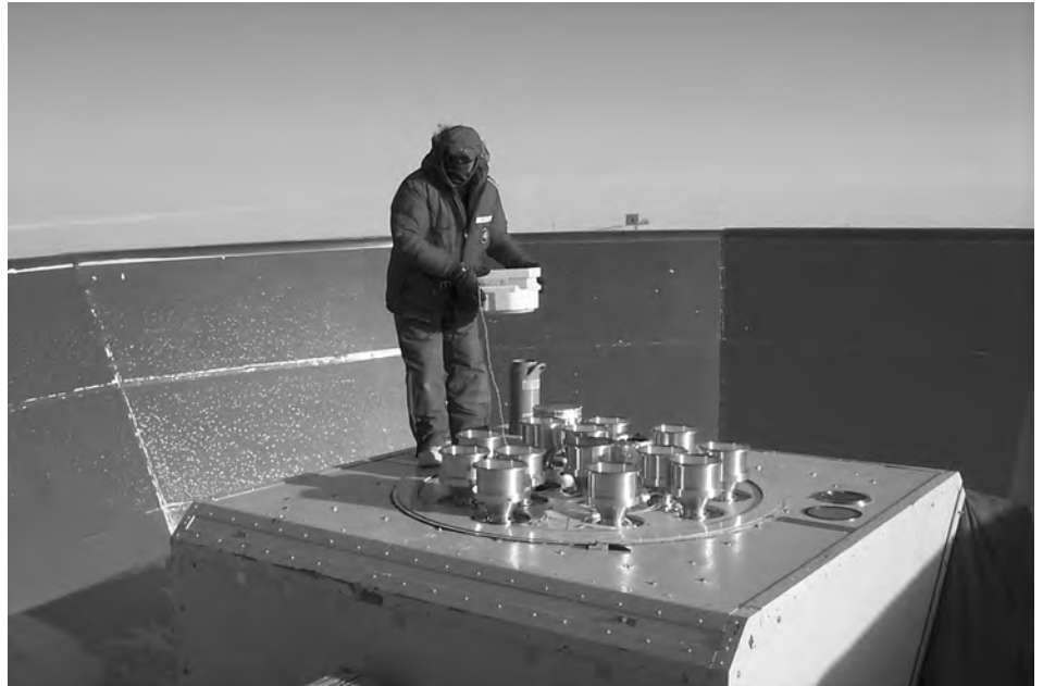
A scientist servicing the Degree Angular Scale Interferometer (DASI) at the South Pole. Each of the small cylinders is a separate detector, and the entire structure is inside a ground shield to reduce scattered microwave “noise” from the surrounding snow. Photo: John Carlstrom
